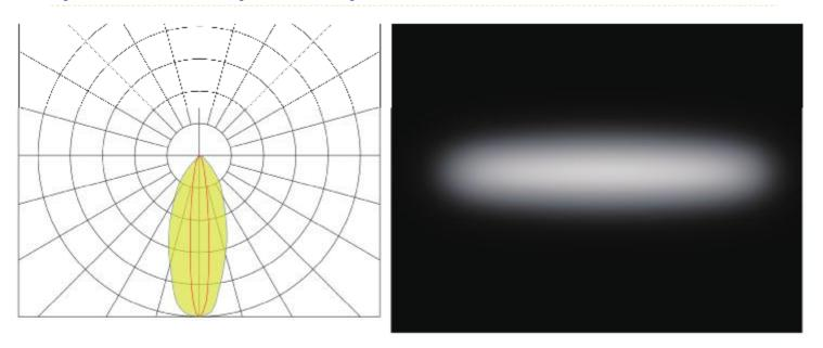
Note:The LED emitter flux is 120lm @350mA
